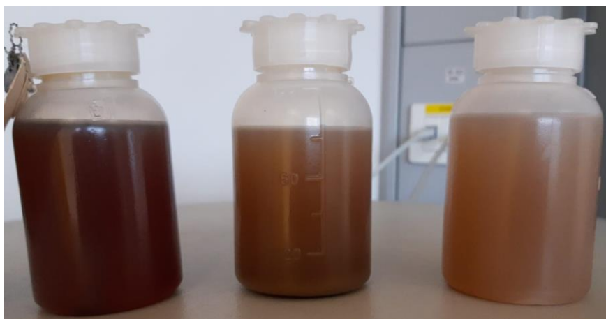
Figure 1: UCO samples used for the HTL and pyrolysis experiments; left: UCO from domestic collection, centre: UCO from restaurants, right: UCO from fast food restaurants.
