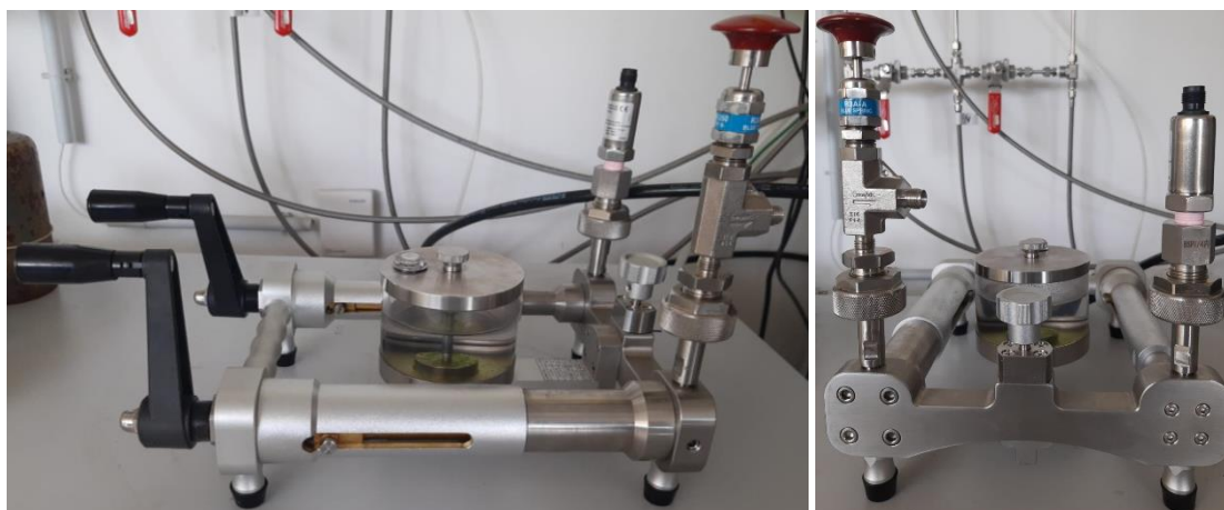
Figure 4: Pressure comparator used for HPRV setting.
