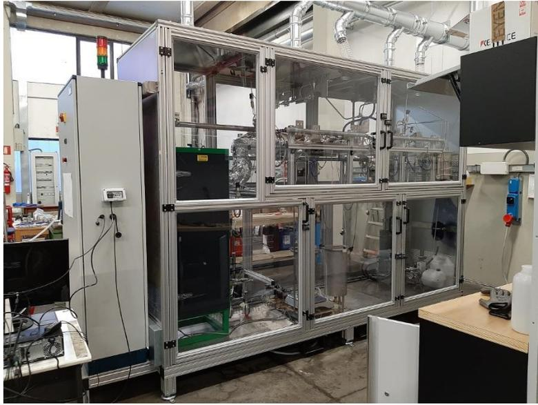
**Figure 21: Continuous hydrothermal liquefaction unit at RE-CORD facilities.**
