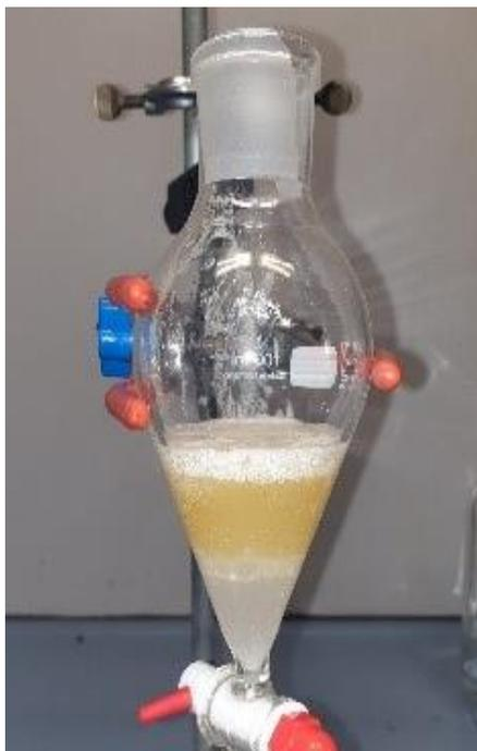
Figure 26: Separation of the heavy and lighter phase for analysis by decanter.
