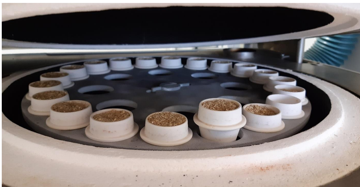
Figure 4: Wheat straw feedstock in LECO TGA 701.
