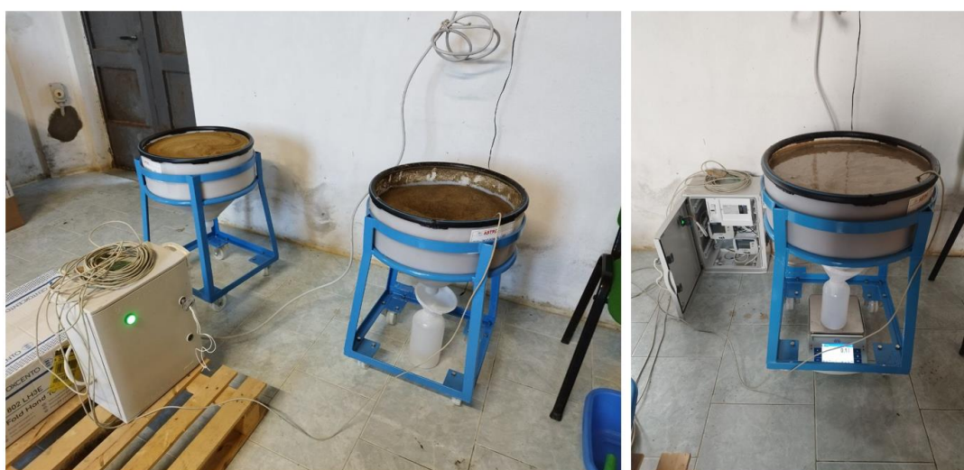
Figure 10 Preliminary wetting test using soil from Terontola field and distilled water.
