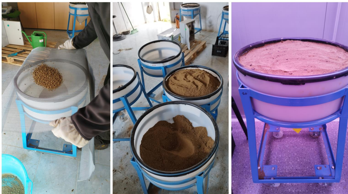
Figure 9 Soil preparation (i.e. soil sieving) before beginning the test within the climatic chamber.
