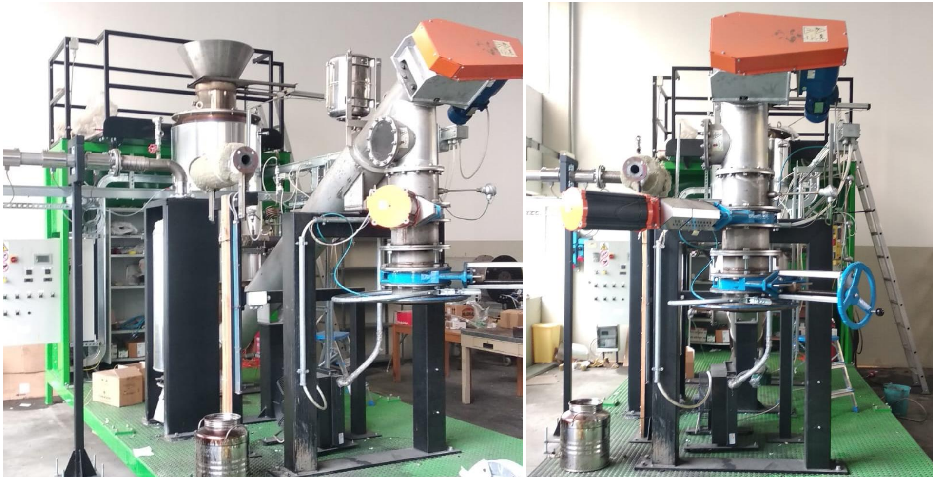
Figure 6: Picture of the new pilot configuration. Insulation removed to show the construction details.
