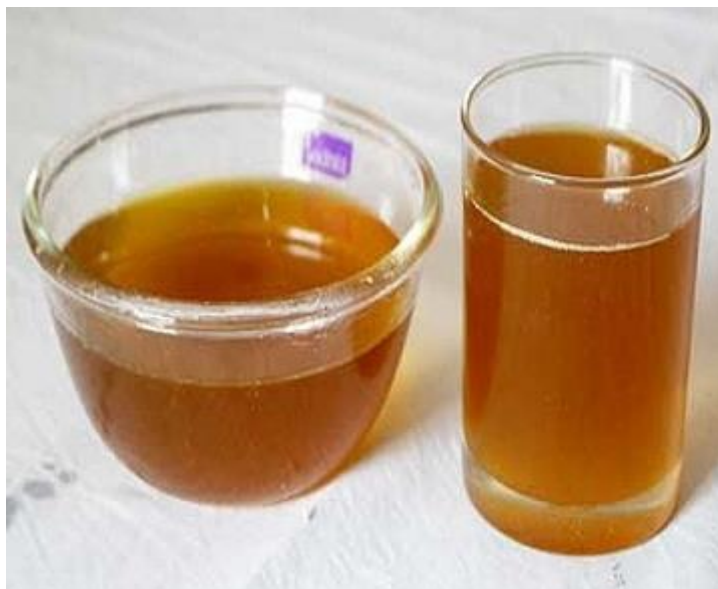
Figure 3. Typical RUCO samples appearance
