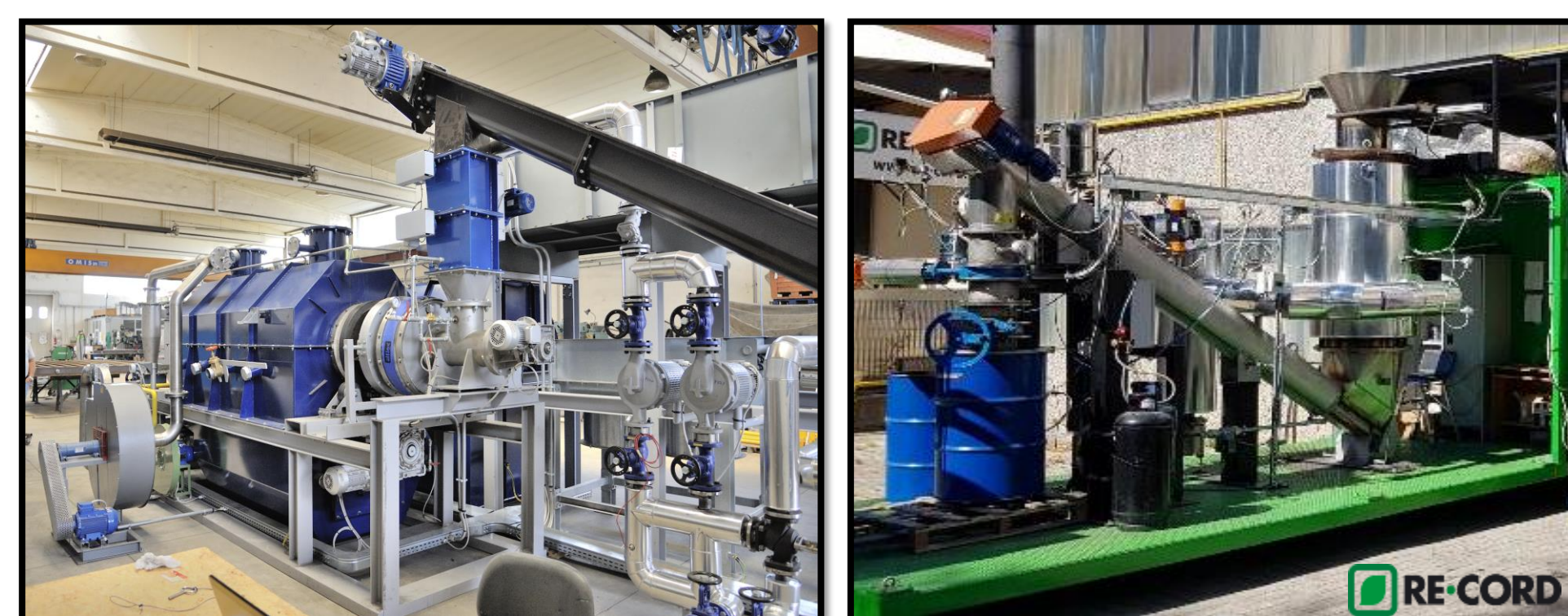
Figure 2: Re-Cord equipment for Biochar production: rotary kiln in the left, CarbOn in the right.
