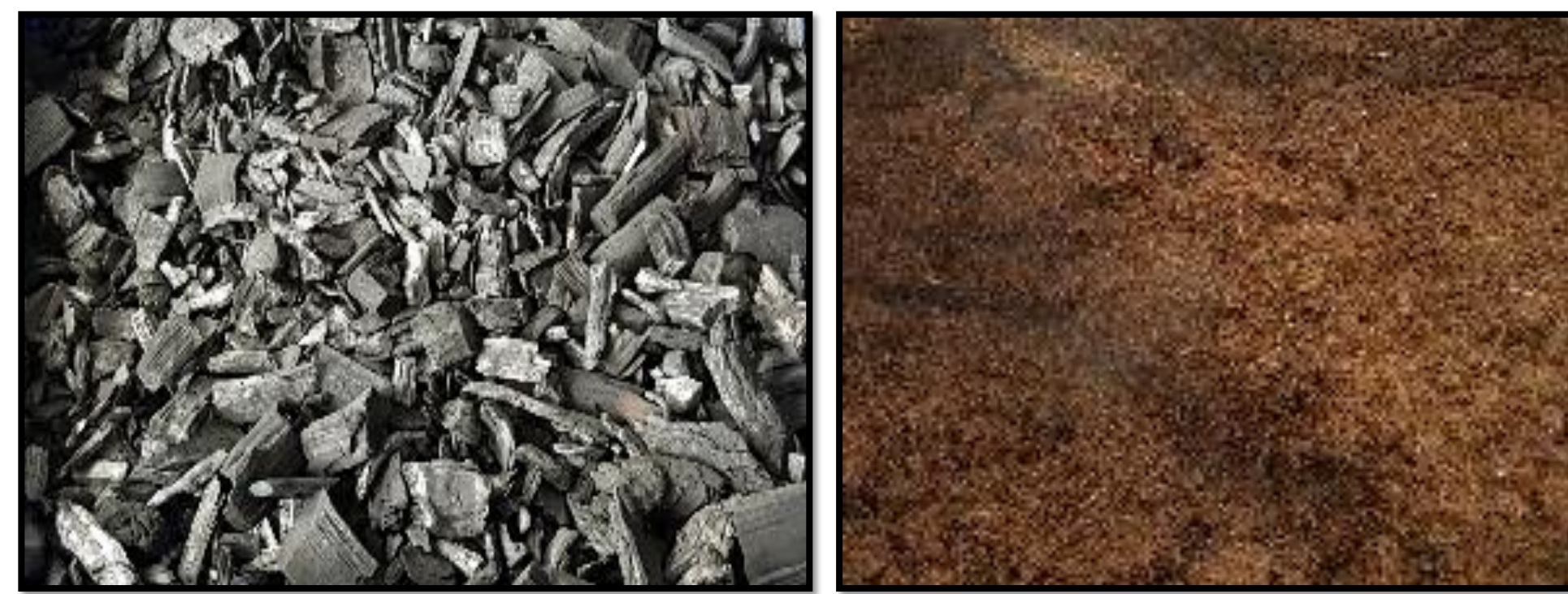
Figure 3: Chestnut Biochar on the left, the solid fraction of digestate from anaerobic digestion (AD) on the right.
